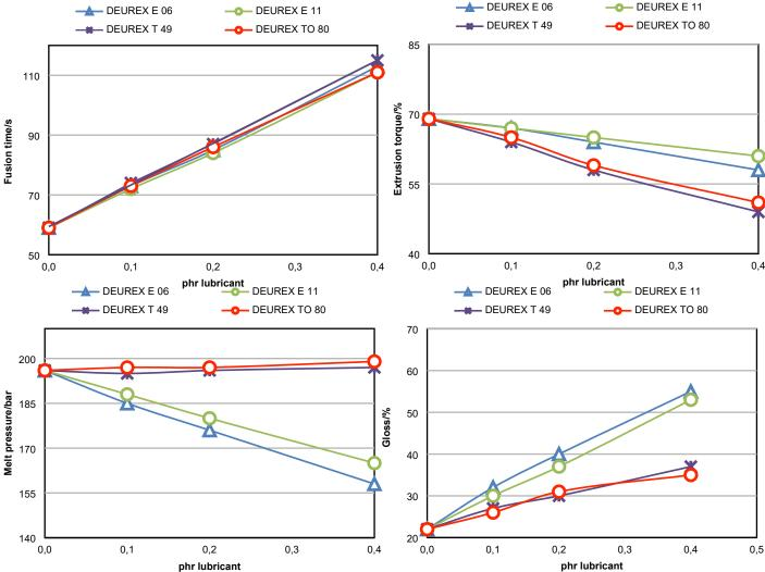
Fig. 1 to Fig. 4 Influence of the dosage of DEUREX® E 06 in comparison to E 11, T 49 and TO 80 on fusion time (Fig. 1), extrusion torque (Fig. 2), melt pressure (Fig. 3) and gloss (Fig. 4)
