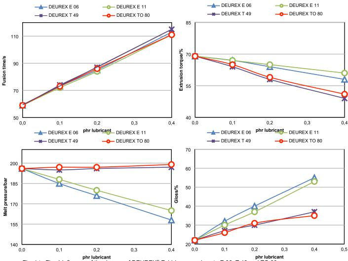
Fig. 1 to Fig. 4 Influence of the dosage of DEUREX<sup>®</sup> E 11 in comparison to E 06, T 49 and TO 80 on fusion time (Fig. 1), extrusion torque (Fig. 2), melt pressure (Fig. 3) and gloss (Fig. 4)
