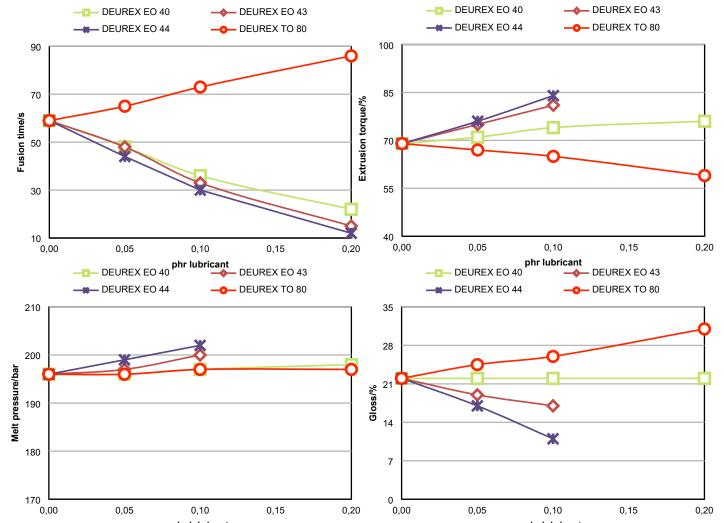
Fig. 1 to Fig. 4 Influence of the dosage of DEUREX® EO 40 in comparison to EO 43, EO 44 and TO 80 on fusion time (Fig. 1), extrusion torque (Fig. 2), melt pressure (Fig. 3) and gloss (Fig. 4)
