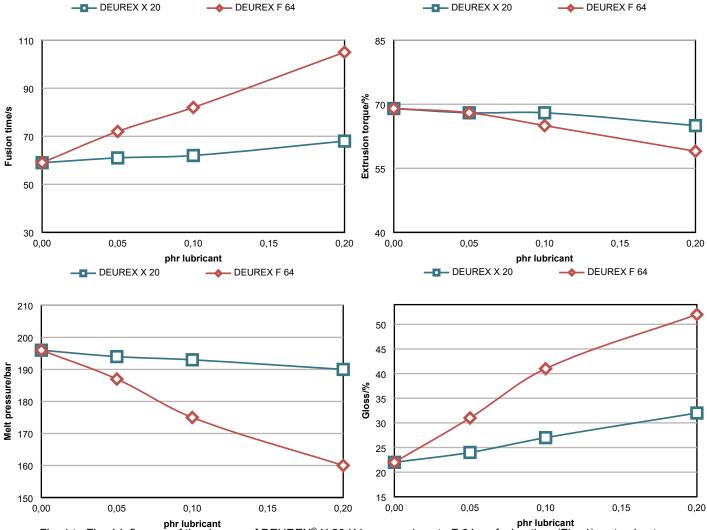
phr lubricant Fig. 1 to Fig. 4 Influence of the dosage of DEUREX<sup>®</sup> X 20 K in comparison to F 64 on fusion time (Fig. 1), extrusion torque (Fig. 2), melt pressure (Fig. 3) and gloss (Fig. 4)
